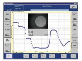
ECV Pro profile of a InP/GaInAsP Laser test structure.
