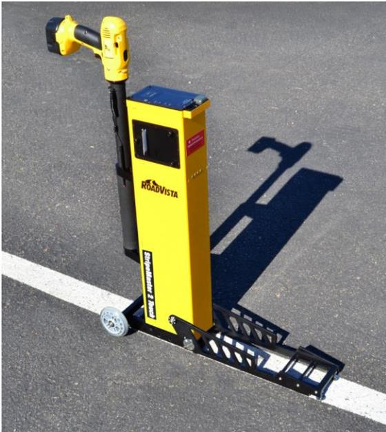
Agencies and contractors require a rapid and efficient way to verify the retroreflectivity of pavement markings. The StripeMaster® Touch series is a highly reliable, field-proven tool for safe and consistent measurement values with minimal operator training.
