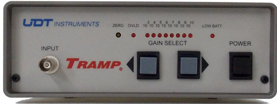
The UDT Instruments TRAMP is a transimpedance amplifier (current-to-voltage) instrument which provides a low input impedance to accurately measure the short circuit current of phototransducers such as silicon and germanium photodetectors, vacuum photodiodes and photomultiplier tubes.
