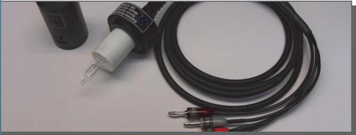
**Gamma Scientific's RS-15 total flux calibration light source is a precision source of total radiant flux, used primarily to calibrate integrating spheres, light measuring instrumentation and as stimuli to measure detection devices. Lamps are available from 5W-200W.**
