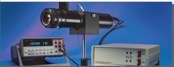
The TIA-3000 Measurement Systems are <u>detector-based</u> <u>absolute standards</u> for various measurements. Off-the-shelf configurations include thermo-electrically cooled silicon and indium gallium arsenide (InGaAs) detectors. Options include high-accuracy photometric correction filters ( $f1^{\circ}$  ~0.8%), flat response filters, trap detectors and ANVIS compatibility filters with field-of-view lenses making the TIA-3000 the standard for any light measurement requirement.
