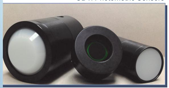
UDTi photometric sensors are designed with advanced photometric filters to simulate the response of the human visual system and match the spectral response of a standard observer. When coupled with an optometer, photometric sensors are used to measure luminous flux (lm), illuminance (lux) and luminous intensity (cd).
