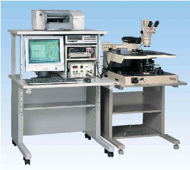
**Manual ESD test of Wafer Level LED**
