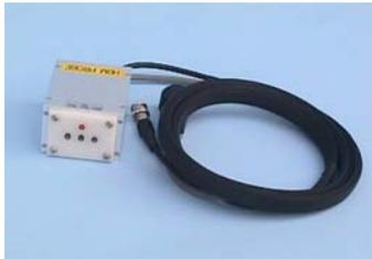
HBM or MM probe for wafer or die test. Model name on case identify HBM or MM probe.
