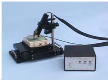
F-CDM probe (P-4F) and control box. Top ground plane size depend on the standard such as ESDA STD or JEDEC STD.
