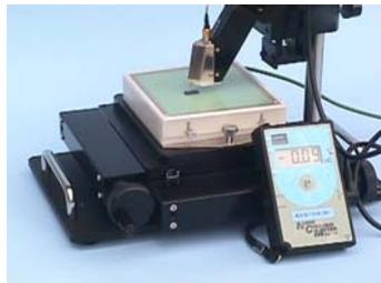
Mobile charge measurement probe (H-1KV) and nano-coulomb meter.
