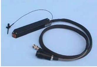
HBM(E-3H) or MM(E-7M) Probe. Type name on case identify HBM or MM.
