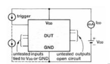
Current Pulse Latch-up Test
