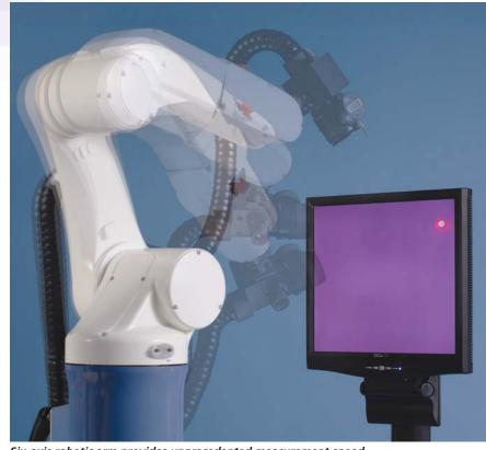
Six-axis robotic arm provides unprecedented measurement speed.
