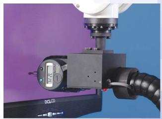
The system automatically monitors – and compensates for – any imperfections in the hemispherical positioning of the display.
