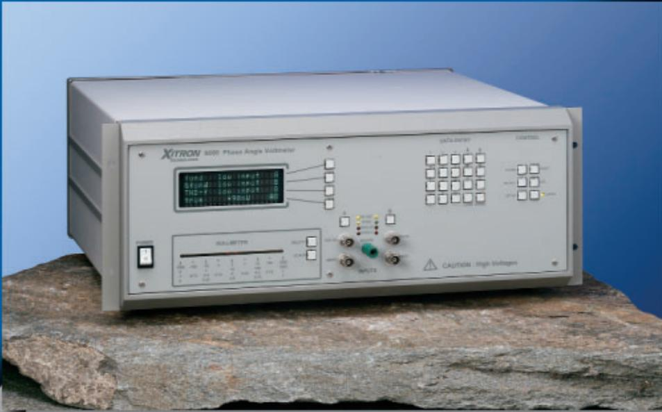
Using the latest digital signal processing technology, the XITRON 6000 PAV delivers true accuracy and versatility. Direct readouts of phase insensitive, phase sensitive and harmonic data are readily obtained at the touch of a button.
