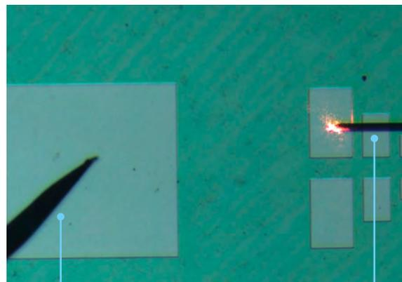
Cantilever/probe for measuring displacement
