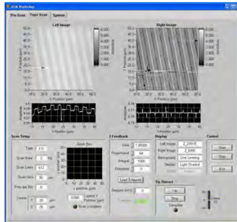
Once all of the steps in the pre-scan window are completed, the scan window is used for measuring images. Scan parameter, Z feedback parameters, and image view functions may be changed with dialogs on this screen.
