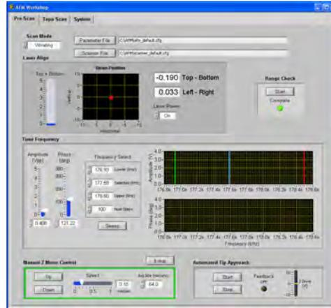
A pre-scan window includes all of the functions that are required before a scan is started. The functions are presented in a logical sequence on the screen.
