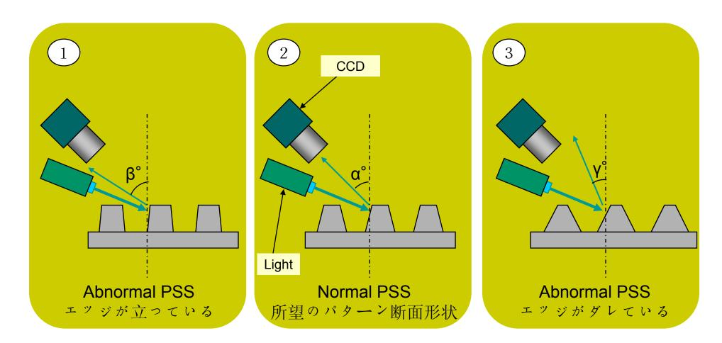
Abnormal PSS (or pattered resist) and normal PSS have different reflect angle and different intensity of scattering light.
