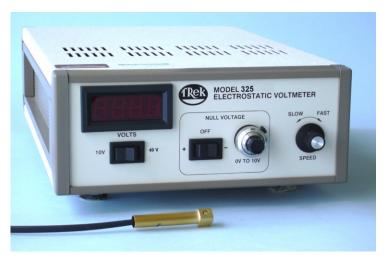
The Trek Model 325 Electrostatic Voltmeter is a versatile instrument used for performing noncontacting electrostatic voltage measurements in applications which include contact potential (surface work function) determination, materials evaluation and electret studies. The Model 325 was specifically designed for high sensitivity applications to allow highly accurate, low noise, noncontacting measurement of electrostatic voltages of 0 to  $\pm40$  V over a wide range of probe-to-surface distances.
