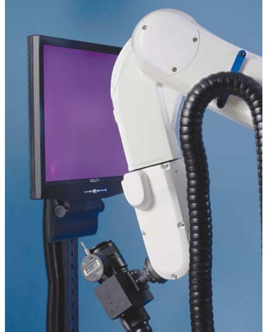
*Perform complete hemispherical measurements centered around any point on the screen.*
