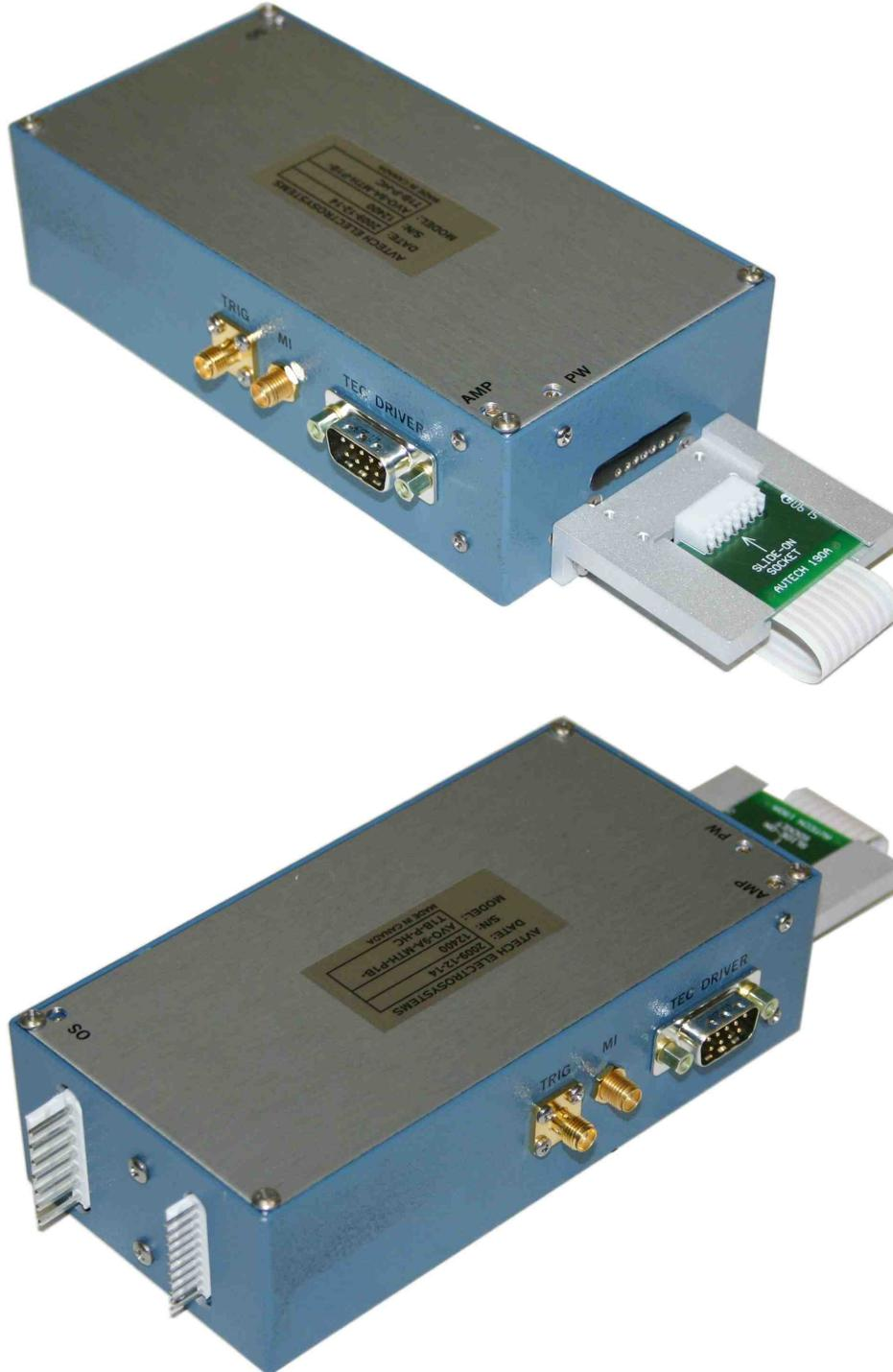
The basic dimensions of the blue module shown in the photo (excluding the connectors and brackets) are 1.67" x 3" x 6", or 42.4 x 76.2 x 152.4 mm.
