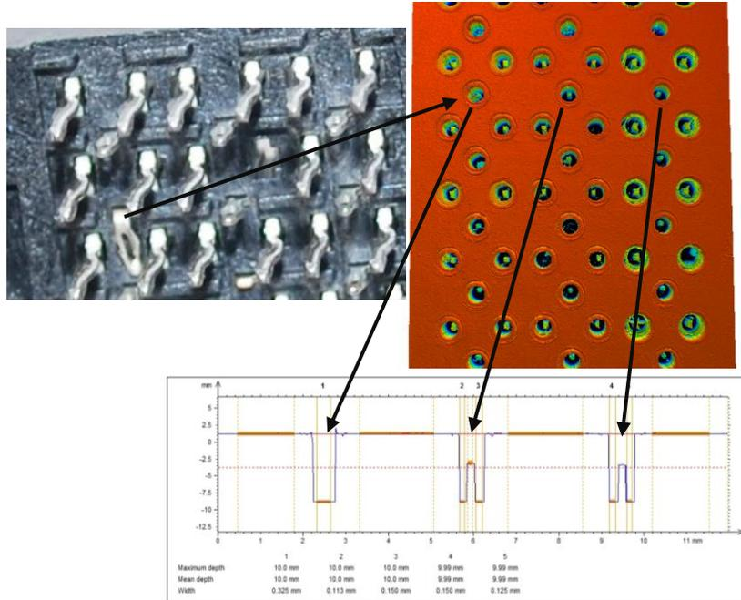
**Bent-Under Connector Pin Defect**
