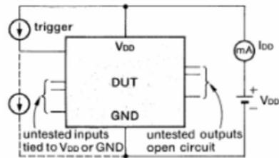
**Current Pulse Latch-up Test**
