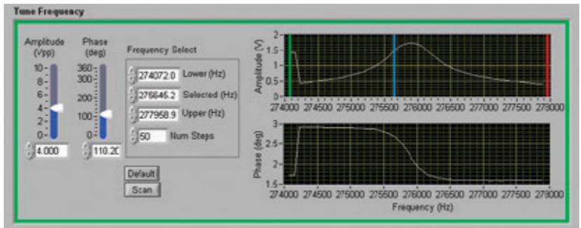
With the window above the resonance frequency of a cantilever is readily measured. Additionally, the phase characteristics of the probe-sample interaction may be captured.
