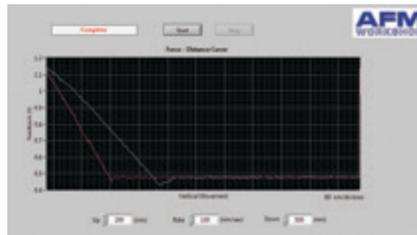
There is a tab for measuring F/D curves in the AFMWorkshop software. Data is exported to a .csv file for analysis in standard programs such as Microsoft Excel™.
