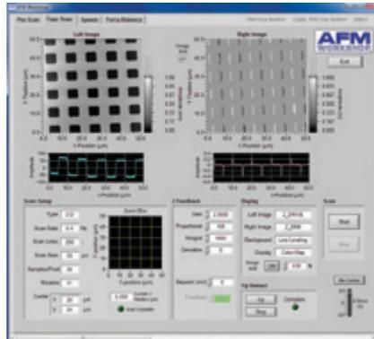
Once the steps in the pre-scan window are completed, the scan window is used for measuring images. Scan parameter, Z feedback parameters, and image view functions may be changed with dialogs on this screen.
