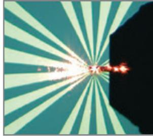
The video microscope is used to locate surface features for scanning. The vibrating mode probe cantilever shown here is 125 microns long. The sample is a reference for conductive mode AFM which has several electrodes that come together in the center.
