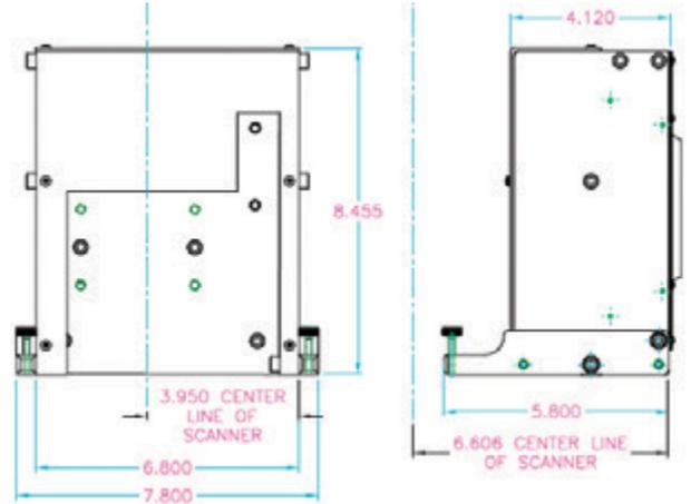
Back and side view of the SA-AFM stage without the AFM/video microscope. The feet at the bottom may be removed if the stage is rigidly mounted to a surface.
