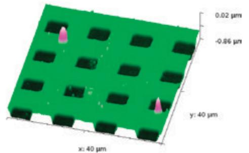
Calibration reference - 40x40x1 micron
