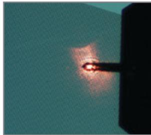
Laser alignment is greatly facilitated with the video optical microscope. With a resolution of 1.5 it is possible to directly visualize the position of a laser spot on the cantilever. The video optical microscope is also used to increase the rate of probe approach. It is possible to estimate the distance between a sample and probe by focusing first on the sample and then on the probe.
