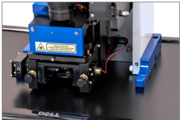
Large objects that will not fit in a traditional stage may be imaged with the SA-AFM. In this example, the monitor of a commercial AFM is being imaged.
