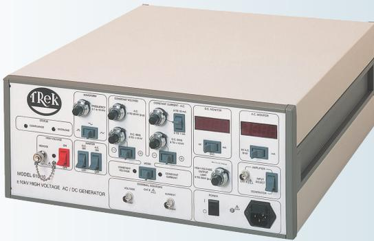
The Trek Model 615-10 is a precision high voltage AC/DC generator and amplifier system used in a broad range of R&D and production applications. In the constant voltage mode, the 615-10 generates constant amplitude waveforms with or without DC bias. In the constant current mode, it generates constant amplitude AC current waveforms, with or without DC bias and in amplifier mode, an analog voltage input connector is provided to apply external AC or DC signals.
