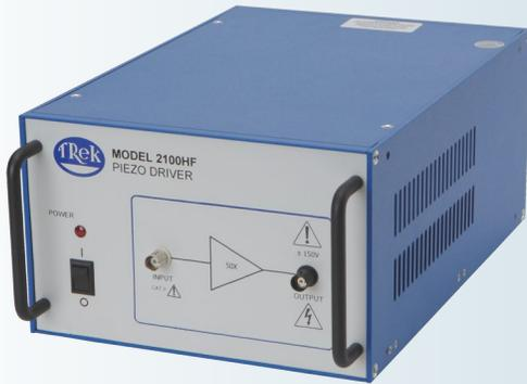
The Trek Model 2100 HF is a high-frequency, high-speed, wide bandwidth amplifier for high power applications. It incorporates an all-solid-state design for highly reliable low-noise operation, thus achieving accurate output response and high slew rates, even in highly capacitive loads. Full power frequency response of the amplifier is essentially flat up to 2 MHz. No overshoot or instability of the waveform occurs due to the amplifier's unique dual feedback feature.
