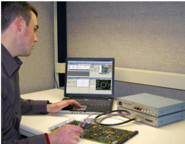
The Huntron Tracker Model 30 is a new compact Tracker designed for use with Huntron Workstation and accessories such as the New [Scanner II](#), the new [Scanner 31S](#) or an Huntron Access Prober. Take advantage of Tracker Signature Analysis capabilities to help you troubleshoot printed circuit board (PCB) faults to the component level and without applying power, saving circuits from possible further damage.
